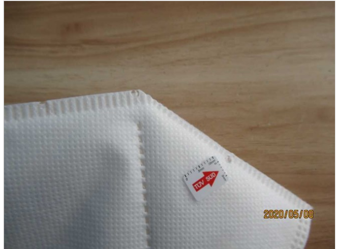
Poor hot-pressing edge
