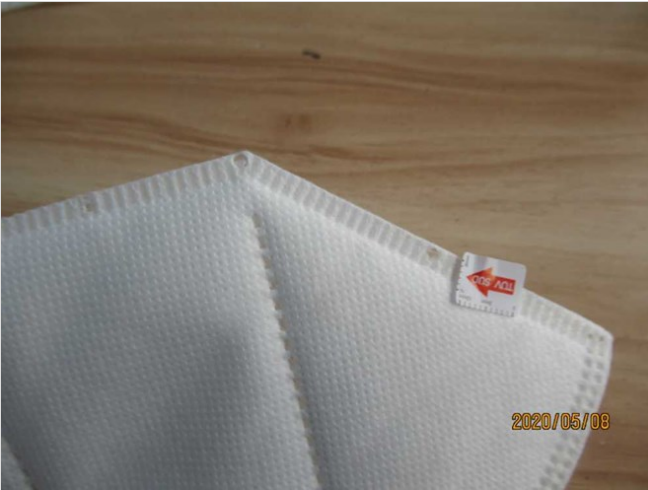
Poor hot-pressing edge
