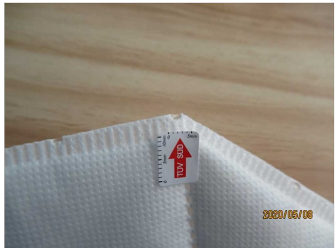
Poor hot-pressing edge
